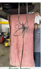
Seen here: balancer completely came off and serpentine belt snapped! Attached is a diagram to show how these two parts work in sync!
